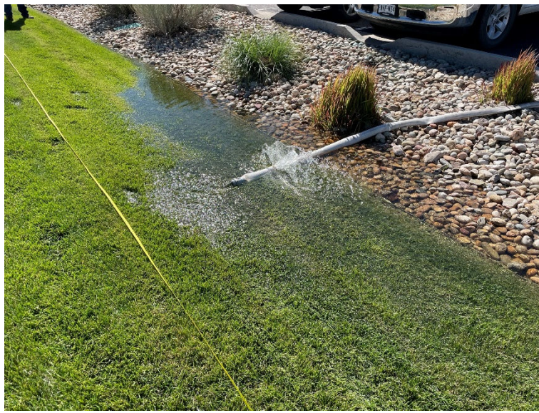
Figure 27. Upstream flow (to the left of the fire hose in the photo) observed during the first SRT at Smith & Smith site
