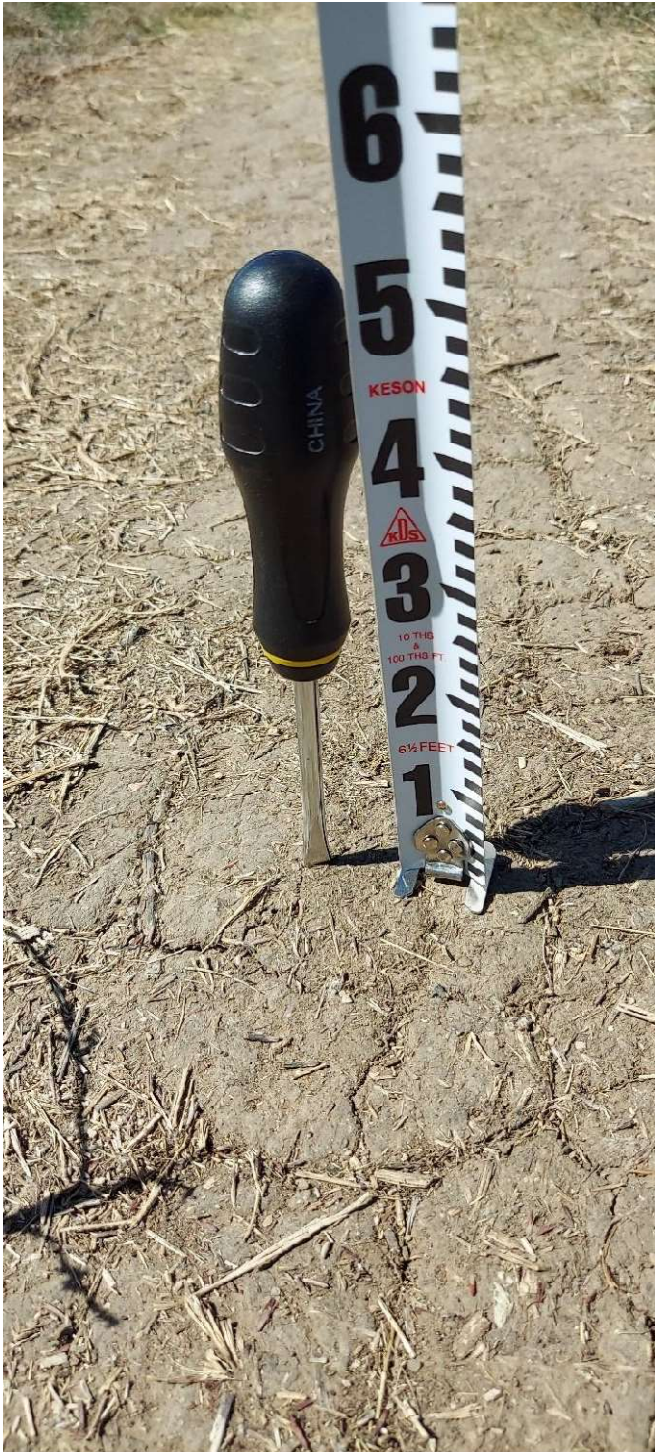
Photo 13 – 10/10/22 (Compaction test along access)
