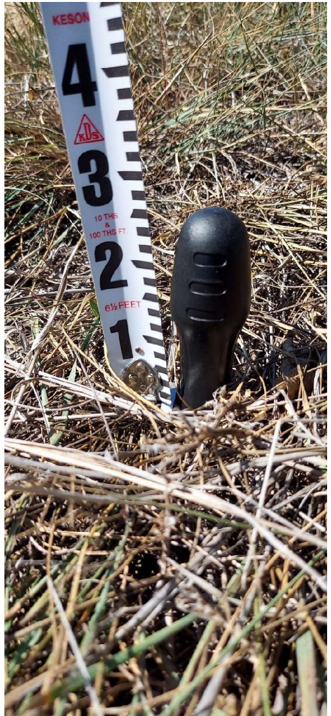
Photo 14 – 10/10/22 (Compaction test outside of access)
